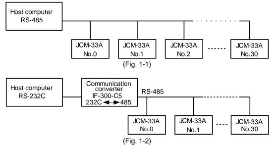
Note: When communication converter IF-300-C5 is used, Modbus protocol is not available. For the Modbus protocol, use a commercially available communication converter.
